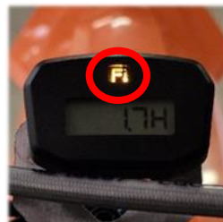
EFI/Fi light visible on original hourmeter
